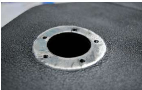
Figure 11: Tank after Drilling
