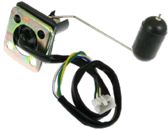
Figure 6: Pre-fit Old Fuel Level Sensor
