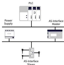
Figure 21: Connection of Vibrosonde via AS-Interface
