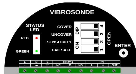
Figure 18: LED Indication on Top Cover
