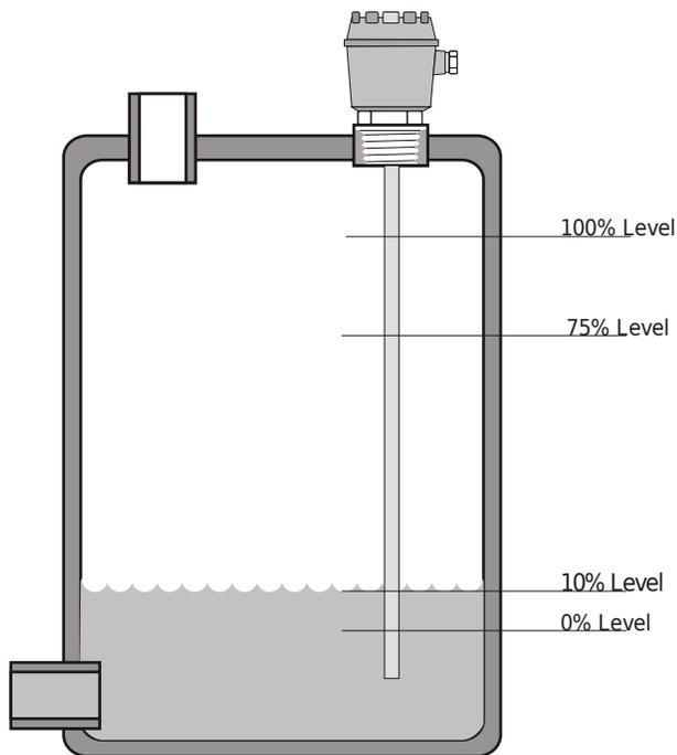
Now, after calibrating and saving (Applying) the 75% level 2 days back, the level is now emptied down to 10%.
