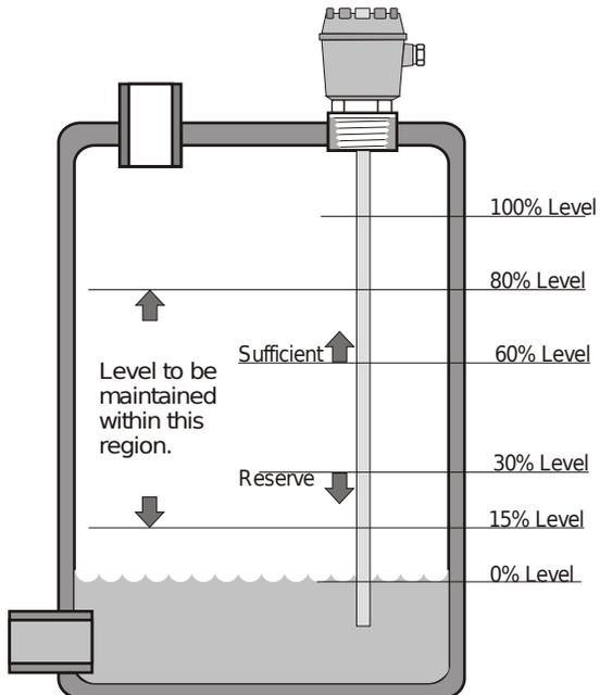
N/C contact of Relay 1 will operate the fill tank valve as long as Level is not filled to 80% from 15%.
