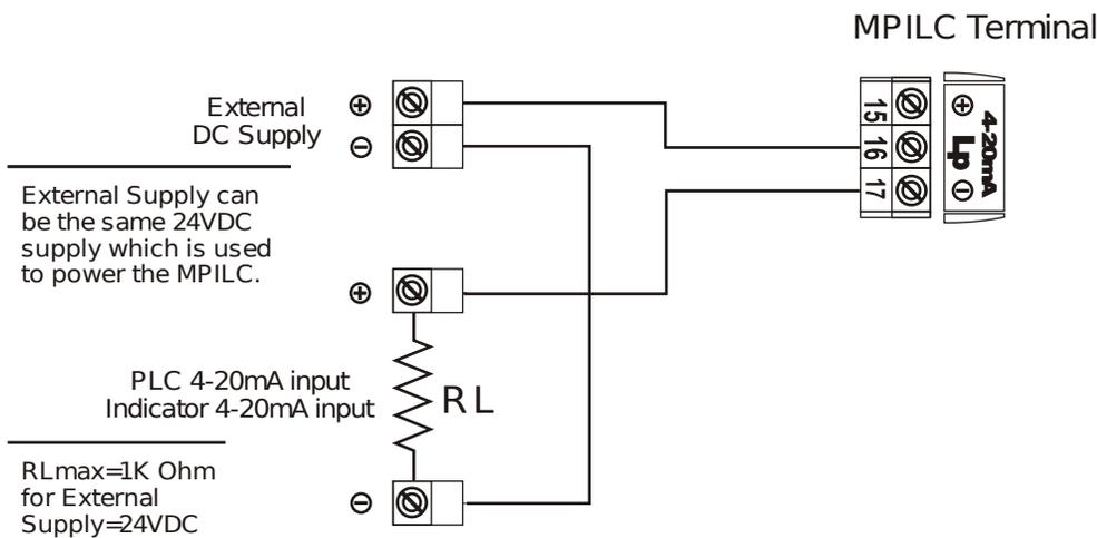
**Loop Resistance = ( Loop Supply Voltage – 4 ) ÷ 0.02 (Ohm)**
