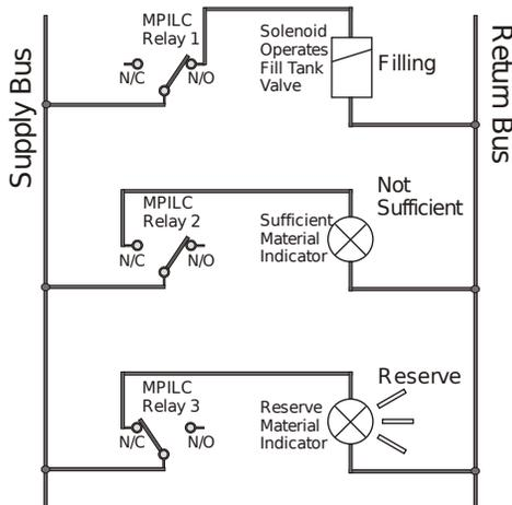
Relay 2: Sufficient Lamp Controller
