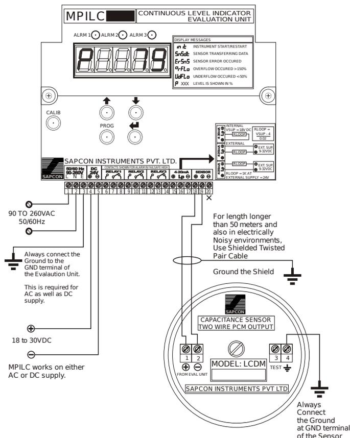
Figure 3: Connection Diagram : Sensor and Power Supply
