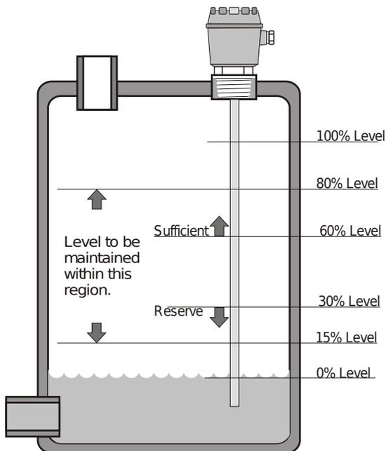
N/C contact of Relay 3 will operate the Reserve Level Indicator Lamp.
