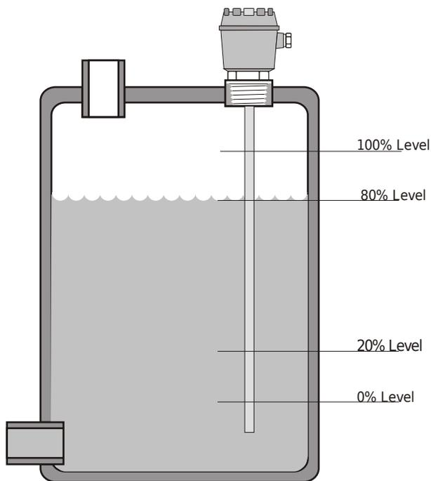
Fill the Tank to desired 80% level.
