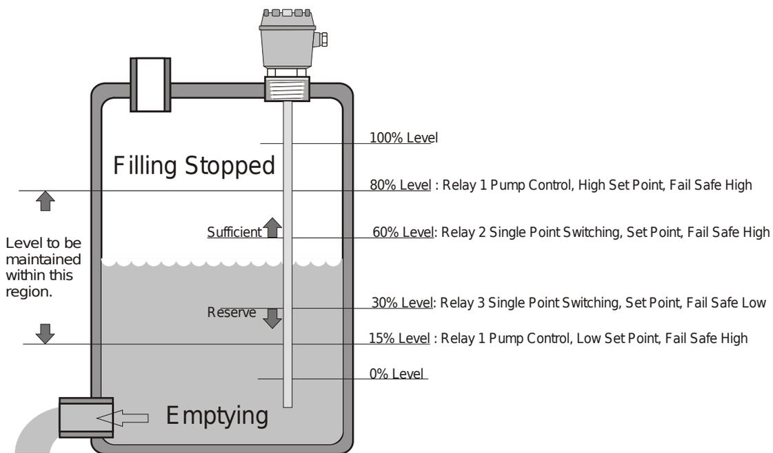
Relay 1: Filling Valve Controller
