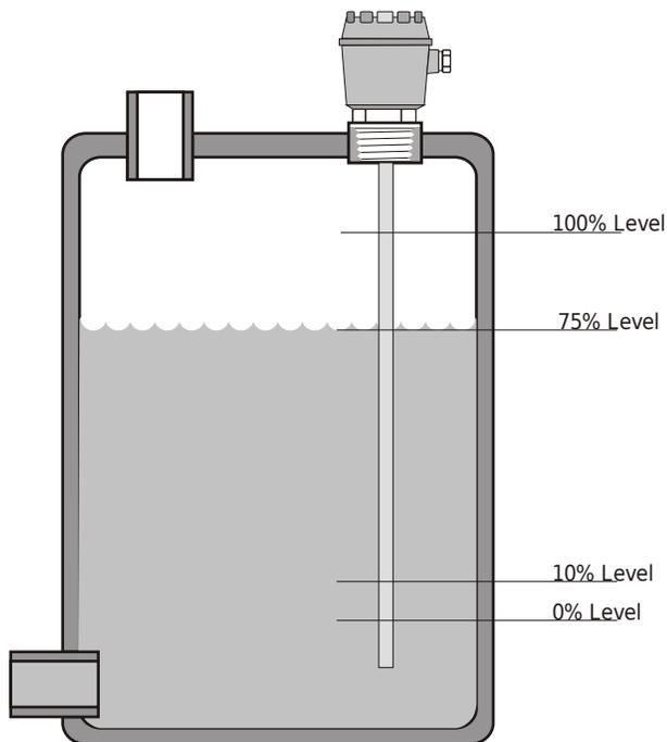
Suppose there is a case that at the time of commissioning of MPILC, the level is at 75%. And this level will fall in next 2-3 days to 10%. In this example it will be shown how to calibrate MPILC over the long intervals of time.
