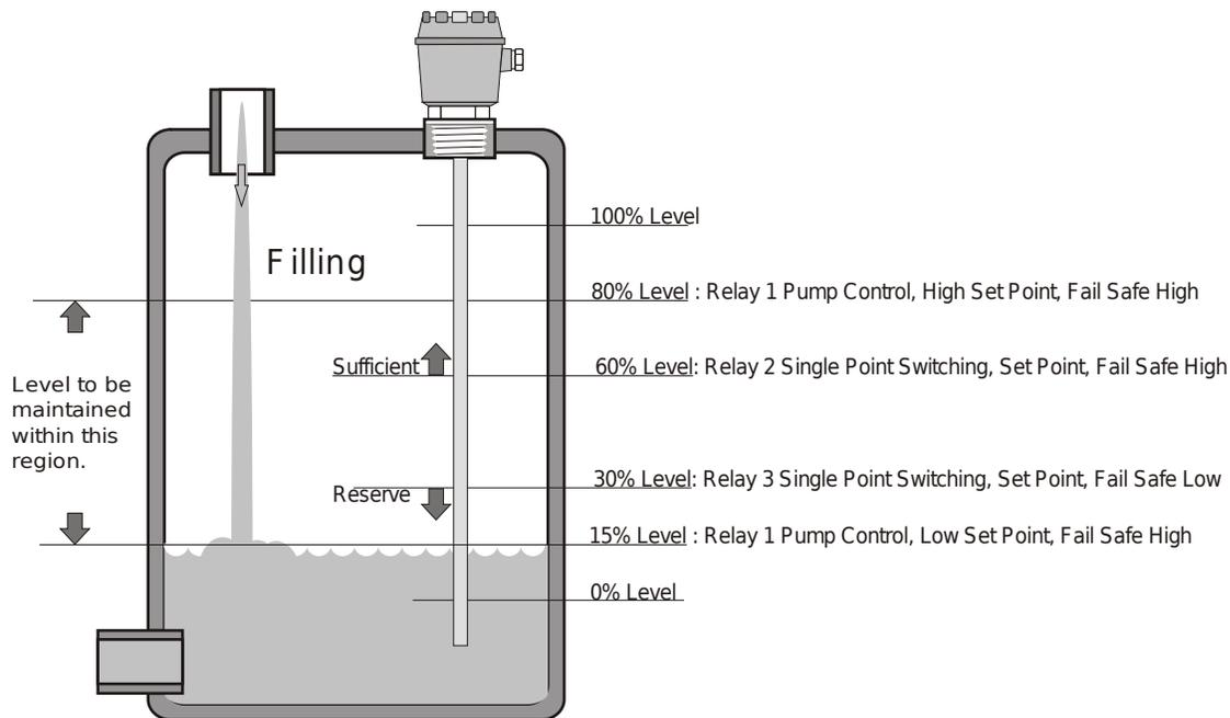
Relay 1: Filling Valve Controller
