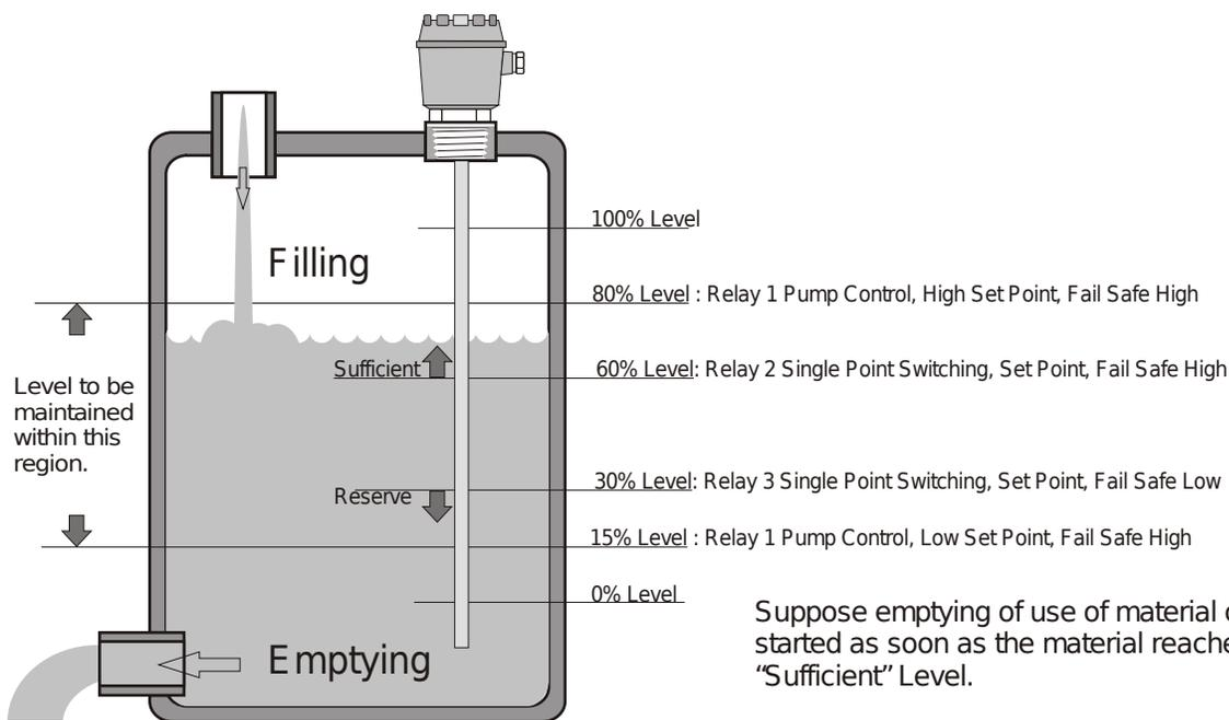
Suppose emptying of use of material can be started as soon as the material reaches its "Sufficient" Level.
