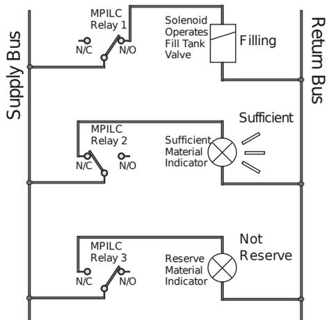
Relay 1: Filling Valve Controller
