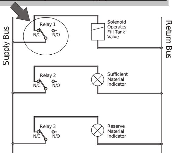
**Solution: Use N/O Contact for Fill operation**
