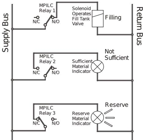
**Relay 1: Filling Valve Controller**
