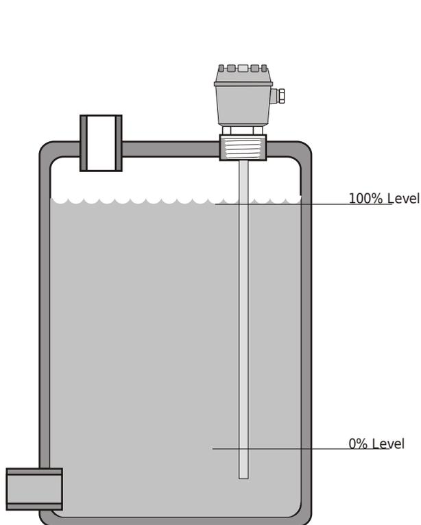
Fill the Tank to desired 100% level.
