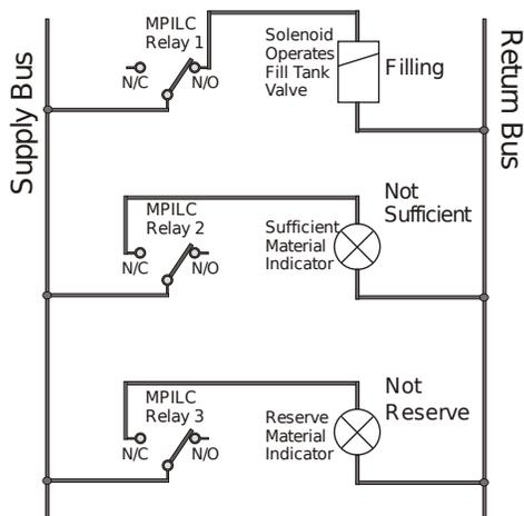
Relay 1: Filling Valve Controller
