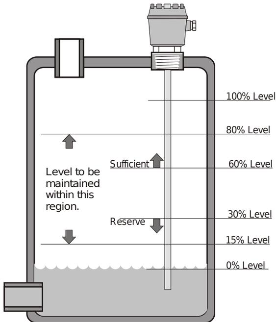
Suppose that it is required in an application to keep a tank filled between the two levels 80% and 15%. And two signals are required when level is above 60% indicating sufficient material and when the level falls below 30% indicating reserve material.
