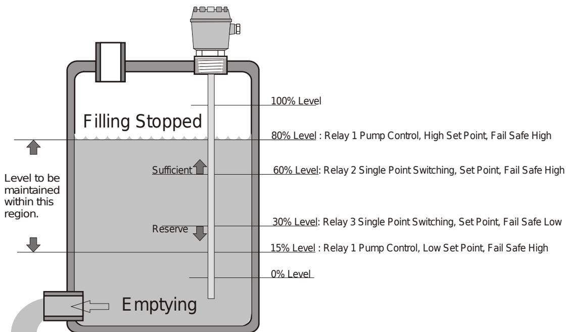
Relay 1: Filling Valve Controller
