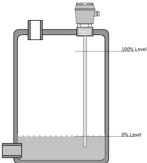
Empty the Tank to desired zero% level.
