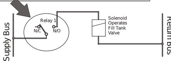
This Solution creates another problem that now the Fill Operation will stop on Level < 15% and will Start on Level >= 80% causing more overflow, with present settings.
