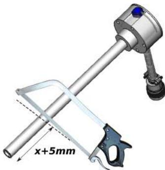
Figure 16: Cutting of Extended Probe Length
